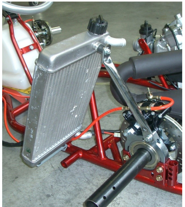
Foto of the frame from the side with the section of the supports for the radiator (radiator mounted)
