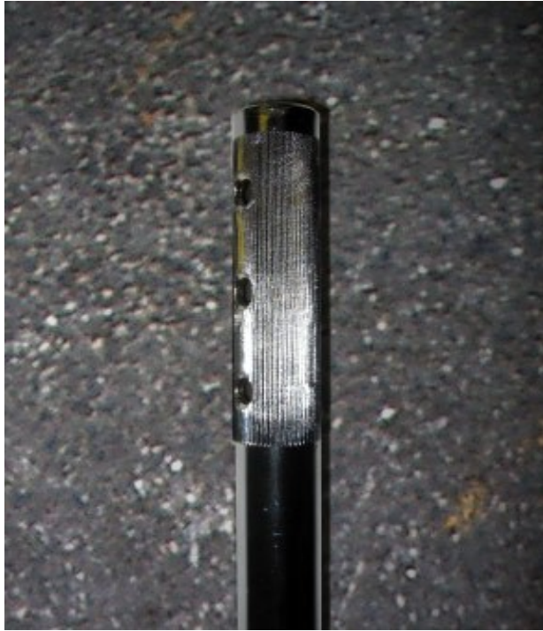
Foto from the steering column with the section with the knurling for the steering wheel hub (knurling according to DIN 82 - RAA1).
