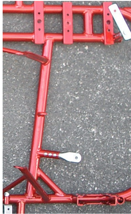
Foto from above of the frame with the section of the two supports for the exhaust system
